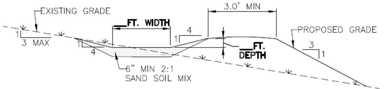
**INFILTRATION BERM DETAIL**
