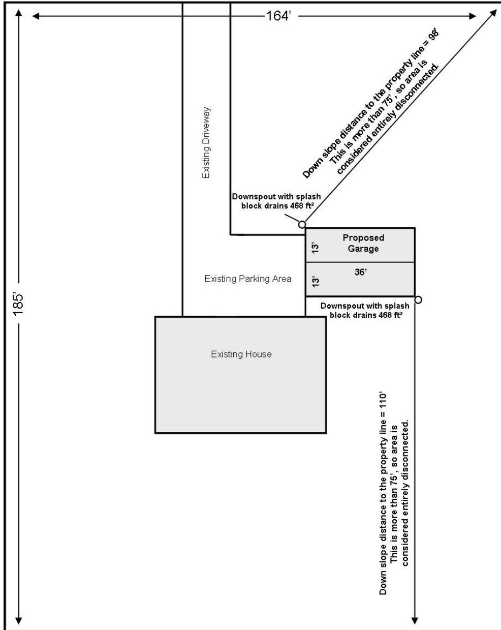
**Step 1:** Determine the area to each disconnected discharge. The area draining to each downspout is 468 ft<sup>2</sup>. This is less than 500 ft<sup>2</sup>, proceed to step 2.
